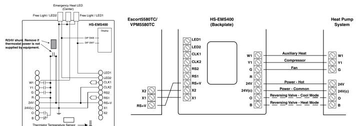
Warning! Do not remove the internal jumper (shunt). Connect to O or B terminal as specified by equipment. Do not connect to both O and B terminals.
