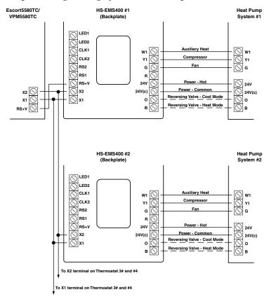
Warning! Connect Escort/VPM RS+V to first thermostat only. Do not remove the internal jumper (shunt).
