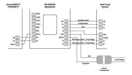
Warning!: Remove the internal jumper (shunt) before connecting the stand-alone transformer. Connect to O or B terminal as specified by equipment. Do NOT connect to both O and B terminals.
